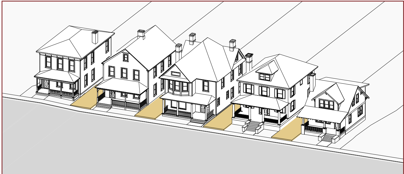
Spacing between houses in Staunton's historic districts may vary depending on the particular street & any new construction should respect the average spacing of the surrounding historic houses.
