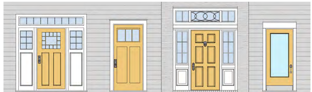
Typical bungalow and American Foursquare doors.
