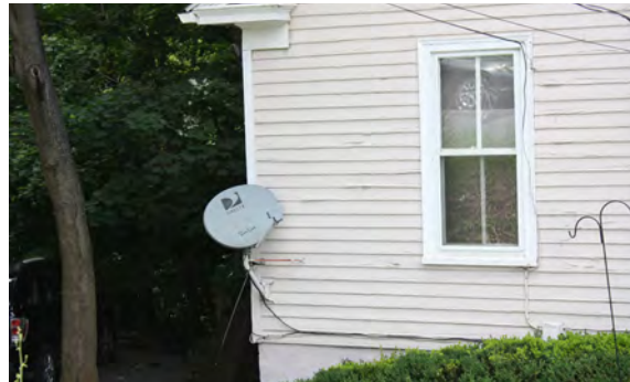
This TV dish is inappropriately mounted on the façade of this historic dwelling.
