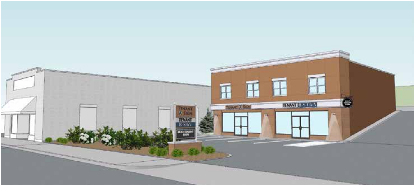
Suggested: Remove mansard and dark siding, paint, add sign band, landscape between sidewalk and parking, incorporate sign in with landscaping
