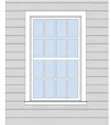
Eight-over-eight sash in 20th c. revival styles.
